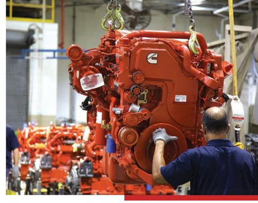
An engine build in process at Kenworth's Chillicothe plant.
