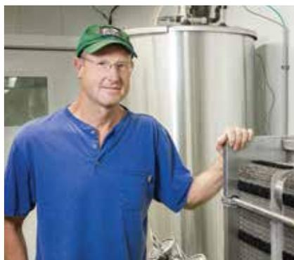
**Bill Deetz**, left, next to the high-efficiency plate cooler that pre-chills the fresh milk before it enters the refrigeration tank
